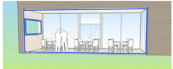
Figure 3: Surface area of openings that contribute to TOTAL NOTIONAL AREA.
